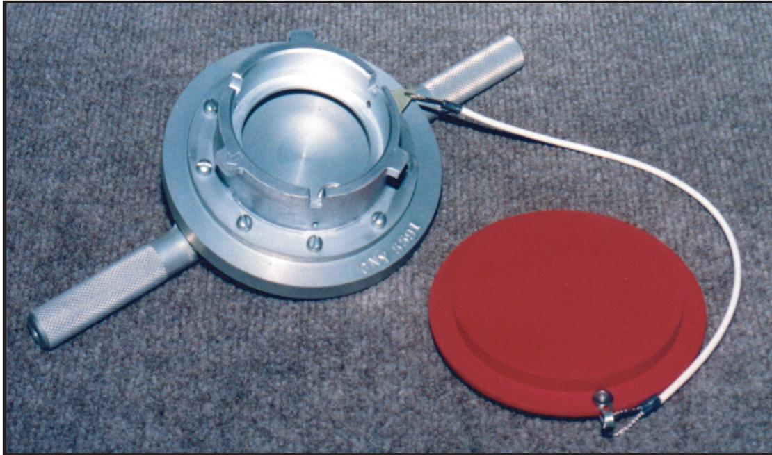
**FOR TESTING LOOSE OR WORN UNDERWING NOZZLE LOCKING LUGS AND NOSE SEAL ASSEMBLIES.**
