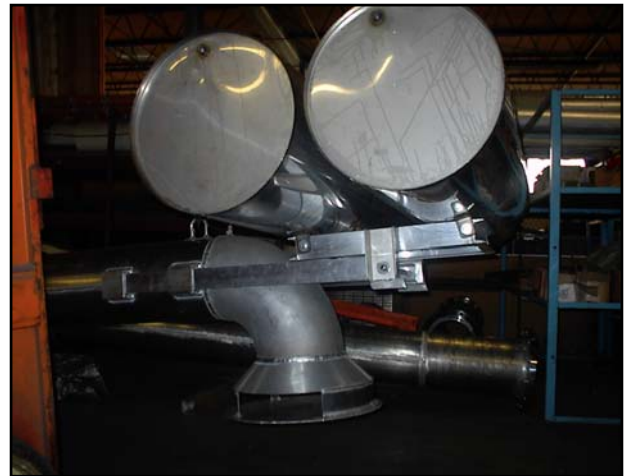
Dual Stainless Steel Float Assembly for 12" Floating Suction Assembly
