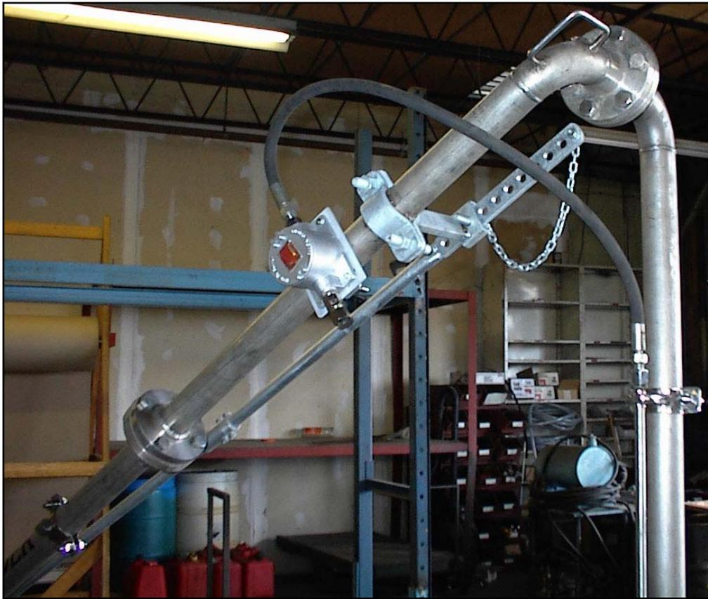
Photographs (close-up) showing, installation (at factory) of top loader with drop tube, filling-in locking system and anti-over spill system with Junction box installation.
