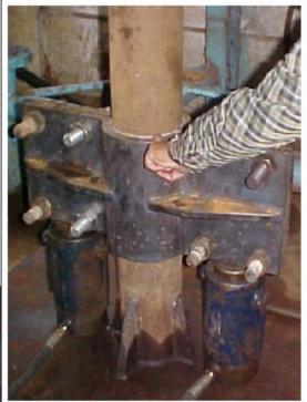
PISTON AREA: 0.7854 X 4.5<sup>2</sup> = 15.90 Sq. Inch. Pr. ATTAINED AT 50 TON LOAD = 50X 2240 / 15.90 = 7044 PSI (487.32 Kg/CM<sup>2</sup>G)
