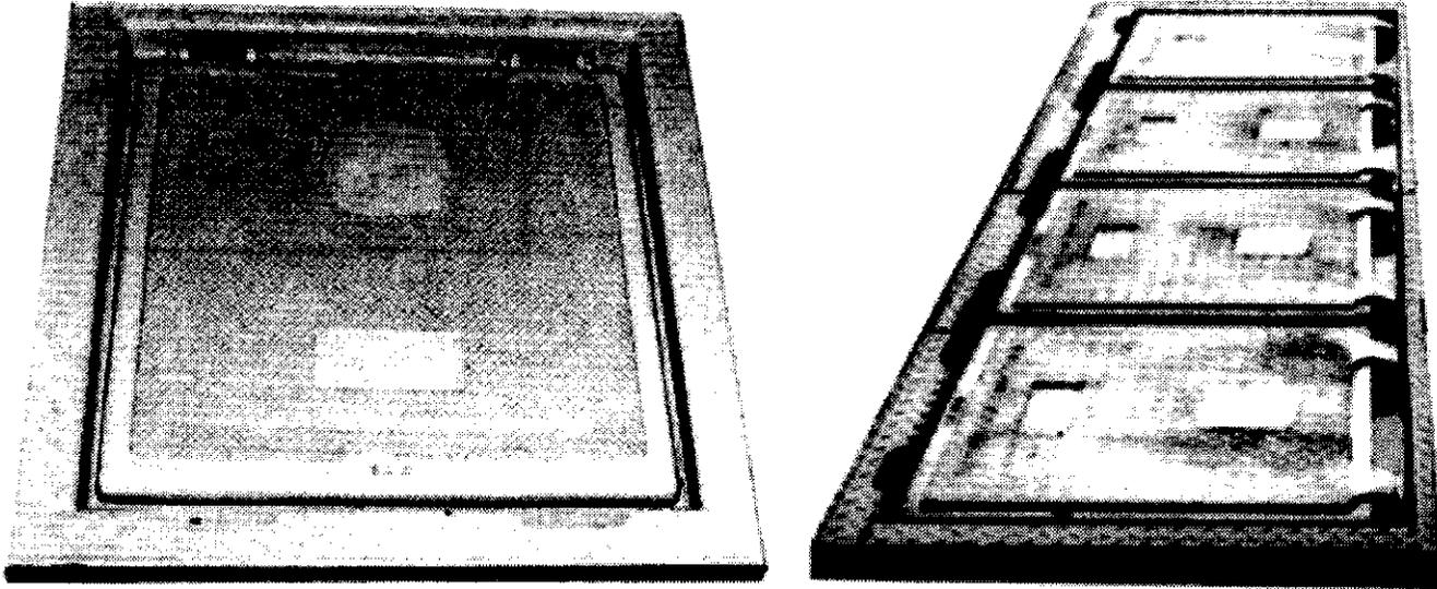
The Model 663PA pit originally was developed as a special hydrant service pit for the JFK International Airport in New York City. The pit consists of a one piece cast aluminum cover assembly and a fabricated carbon steel frame and shell having a 24 inch (610 mm) nominal square inside opening with an open bottom.
