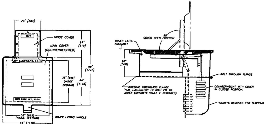
The Model 7038 pit consists of a two-piece cast aluminum cover assembly and a one-piece molded fiberglass shell. The standard pit is supplied with open-bottom shell for access manway into underground vaults. The main cover is hinged and counterweighted for ease of opening to expose a large square 38 inch opening.
