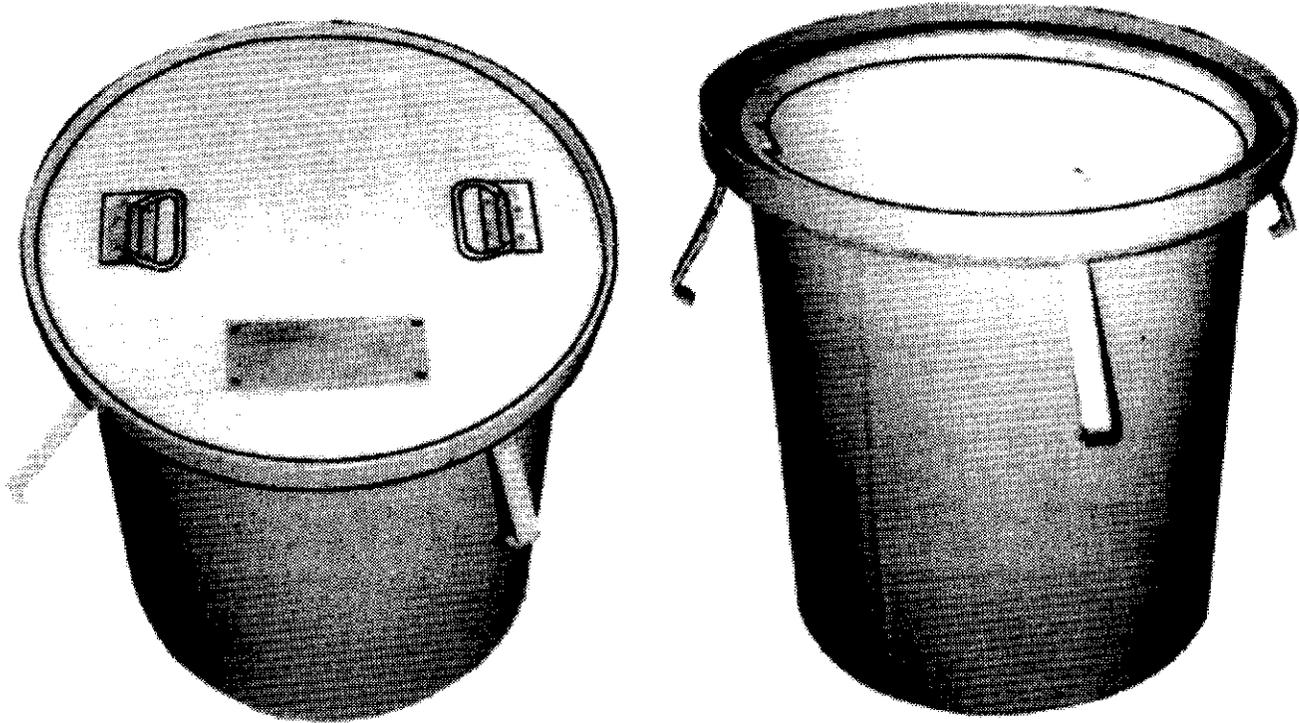
The standard Model 1723FT pit consists of a one piece, skirted, drop-in type, cast aluminum cover assembly, cover gasket and a fabricated carbon steel frame and shell, having a 19 inch (485mm) inside diameter with an open bottom.
