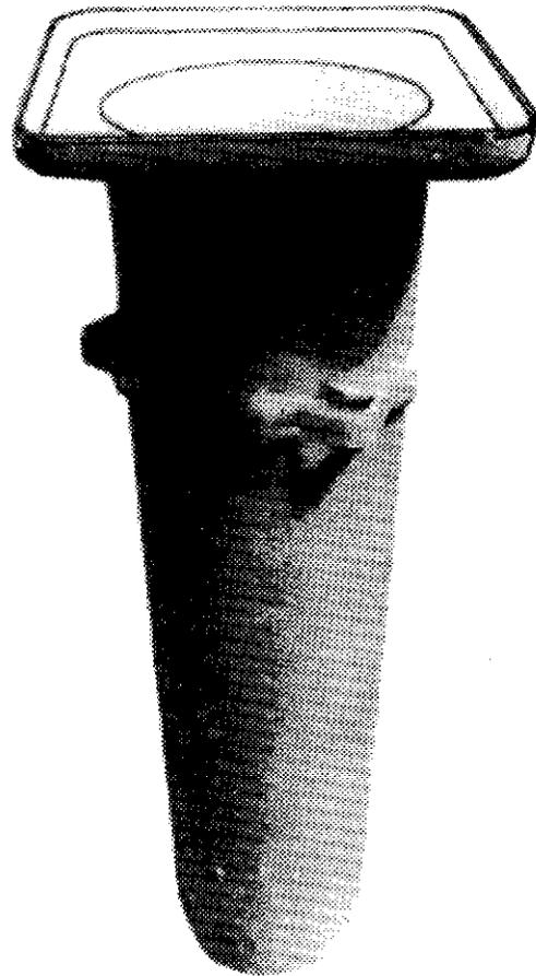
The standard Model GD-360-10 pit consists of a one piece cast aluminum cover assembly and a one piece molded fiberglass shell having a 9 inch (230 mm) nominal inside diameter, with a 10' ground rod and cable.
