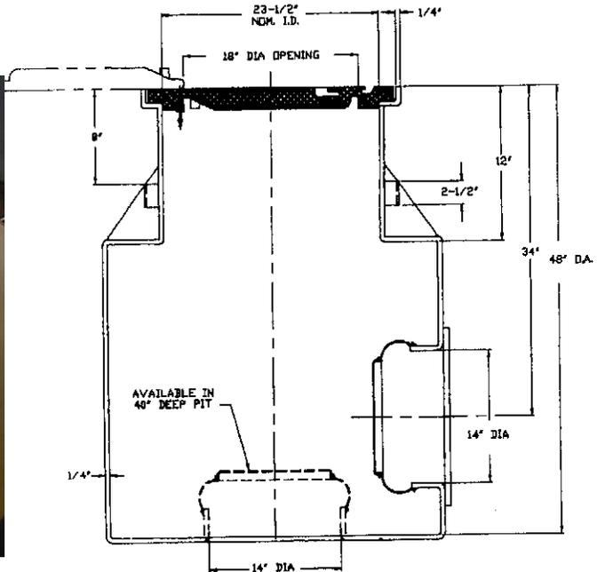
The standard Model 1480 pit consists of a two piece cast aluminum assembly and a one piece molded fiberglass shell, having a bottom or side entrance, pipe collar, flexible fuel-resistant boot type seal, and stainless steel clamps.
