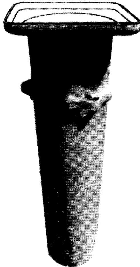
The standard Model 938-UP pit consists of a one piece cast aluminum cover assembly and a one piece molded fiberglass shell having a 9 inch (230 mm) nominal inside diameter.
