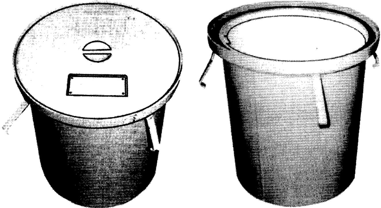
The standard Model 800 pit consists of a one piece, twist-lock, cast aluminum cover, cover gasket and a fabricated carbon steel frame and shell, having a 19 inch (485mm) inside diameter with an open bottom.
