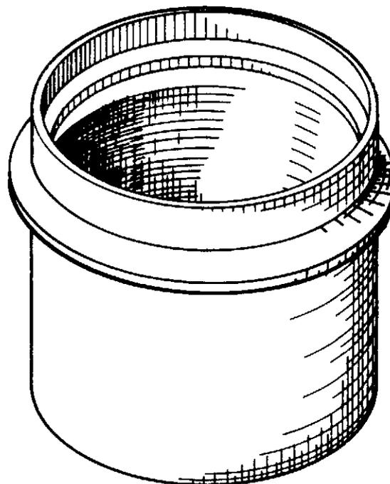
The standard Model 1462-A pit consists of a two piece cast aluminum cover assembly and a fabricated carbon steel frame and shell having an open bottom entrance.
