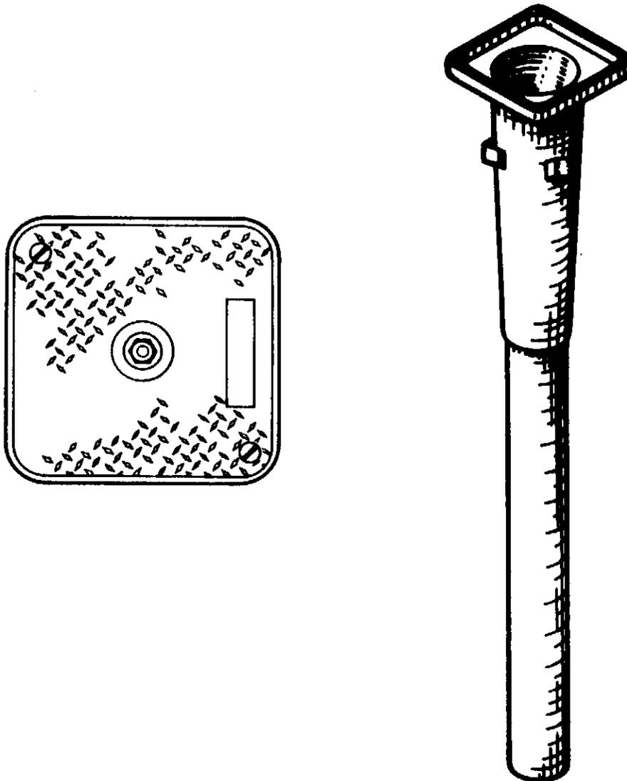
The standard Model GD-360-CB pit consists of a one piece cast aluminum cover assembly and a two piece shell consisting of molded fiberglass and a lower galvanized steel tube.
