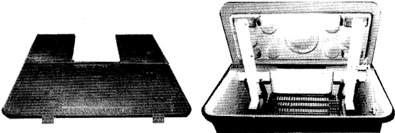
The standard Model 9000 pit consists of a three piece cast aluminum cover assembly and a one piece molded fiberglass shell. The shell entrance(s) can be located in bottom, sides or ends, depending upon application. The main cover is hinged and counterweighted for ease of opening to expose a large rectangular opening.
