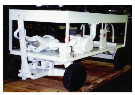
Unit completely assembled. All main product piping of welded aluminum. Entire unit finished with two (2) coats of white epoxy paint. The unit does not include optional additive storage tanks.
