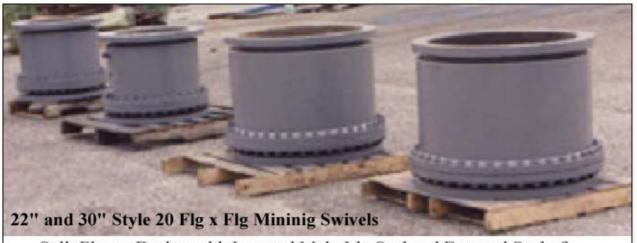
Split Flange Design with Inverted Main Lip Seal and External Seal of PTFE with Viton® insert, Special Lubricant and Heavy-duty Load Bearing Raceways. This units were designed, manufactured, tested, and installed for a South American Foundry in 2001.
