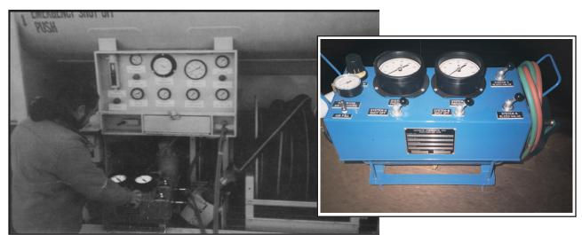
Maintain performance and save time by testing pressure gauges in the field.
