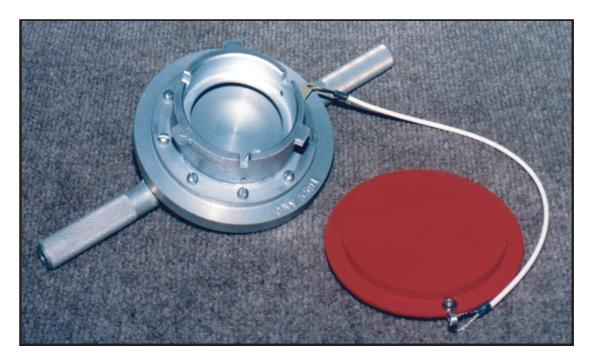
FOR TESTING LOOSE OR WORN UNDERWING NOZZLE LOCKING LUGS AND NOSE SEAL ASSEMBLIES.
