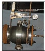
4" Collar Dual Release SBC under testing. Manual release test conducted for successful break-aways. Sizes: 3", 4", 6", 8" and 10" x Class 150 has been tested for GNY Job Number: FB1414.
