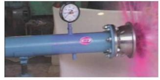
6" Shear-Pins SBC **Hydro Pressure Break Away testing.** A red color water as a visual indicator showing a successful break-away.
