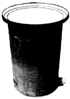
The standard Model 1463FM pit consists of a two piece cast aluminum cover assembly and a one piece molded fiberglass shell, having a bottom entrance, pipe collar, flexible fuel-resistant boot type seal, and stainless steel clamps.
