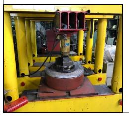
The cover assembly (part numbers 6533774 and 6533772(H) is under load test guarantee to withstand a single 200,000 pound (90720 kg) load applied over a 200 square inch (1290cm2) tire footprint area placed anywhere on it (1000psi (70.3kg/cm2) rating). This represents a 4 to 1 safety factor.
