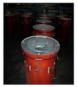
The standard Model 1463WR pit consists of a two piece cast aluminum cover assembly, Hinged-Block and a one piece molded fiberglass shell, dual seals (sealing outer-cover and inner-cover) having a bottom entrance, pipe collar, flexible fuel-resistant Buna-N boot type seal, and stainless steel clamps. Flexible Buna-N boot provides vertical and horizontal movement. Compliance with JIG Bulletin 90.
