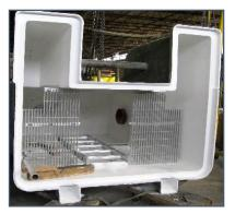
The standard Model 9000 pit consists of a three-piece cast aluminum cover assembly & a one-piece molded fiberglass shell. The shell entrance(s) can be located at the bottom, on the sides and/or even at the ends, depending on the application. The main pit cover is hinged and counter-weighted for ease of opening to expose a large rectangular opening.
