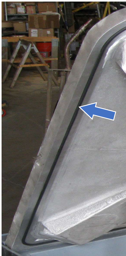
Water-Resistant O-Ring Seal Gasket Installed on Main Counter-Weight Opening Cover (Model 8000WR)
